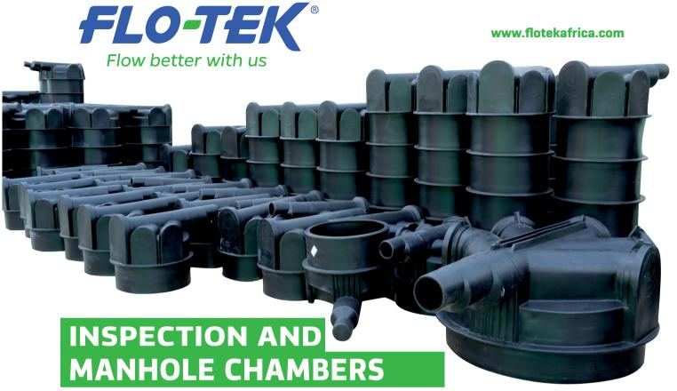
Flo-Tek manhole/inspection chambers are made of virgin UV stabilised polyethylene (PE) material and are intended for use in underground drainage and sewerage systems. The specially designed external ribs give additional strength to the product and at the same time act as an uplift prevention system against a high water table.
