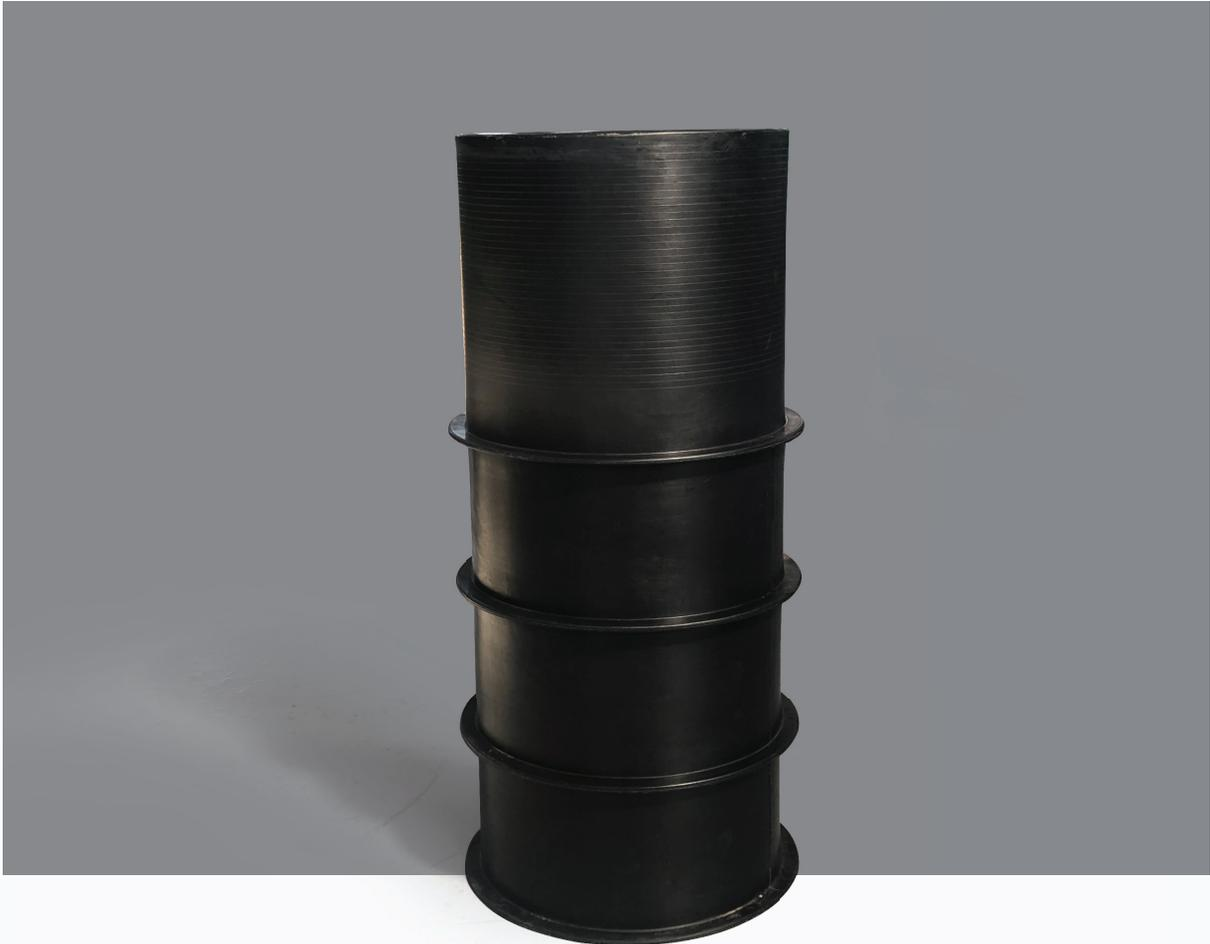
**FLO-TEK** Connection Chambers are manufactured with different sizes and characteristics. Chambers are available as multi-piece or single-piece units. Inlet and outlet connections of desired number can be made with a simple drill at desired diameter and height. The connections can be sealed watertight with gaskets or PE welding. Light weight but strong, does not require heavy construction equipment, can be carried manually, reducing time and installation costs.
