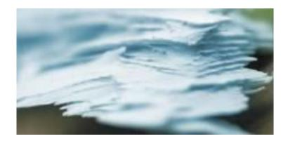
These images above show the laminar structure of PVC-O pipes
