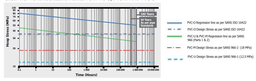
From the 50-year failure stress the Minimum Required Strength (MRS) is determined and the Design Stress ( $\sigma_s$ ) by applying a Design Coefficient (safety factor) (C):
